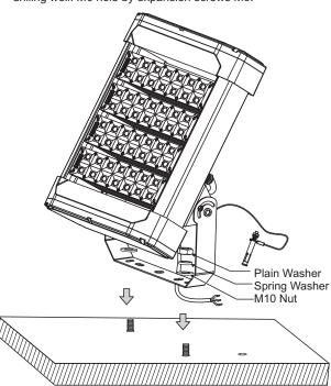
Connect the power wire and make insulation and water-proof processing. Please look at detail A/B at the wiring place. (please connect wires as per appropriate color of power cords as shown in A/B diagram.)
