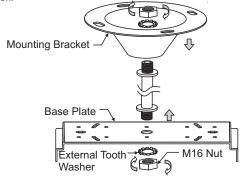
Pass the power supply wire through base plate, suspender and mounting bracket as the sketch shows.
