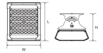
Mounting height≥8m, the maximum projection area of undergoing wind:  $L(m) \; x \; W(m) \; x \; 0.5$
