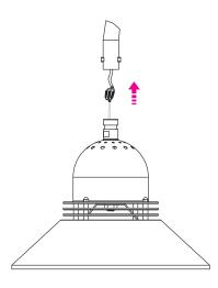
Step 3: Tighten the light with screw by wrench and make sure the light is firm.
