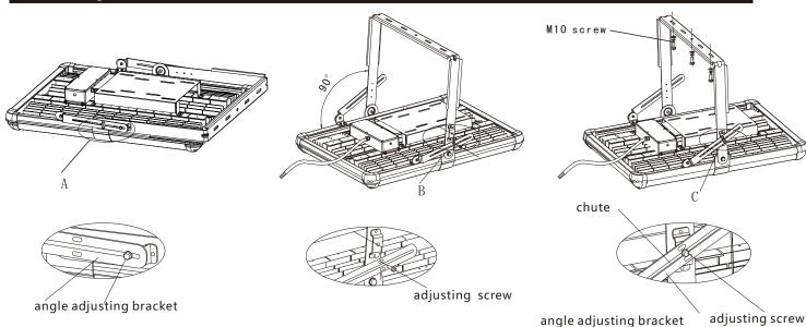
Loosen the adjusting screw , lock the screw as diagram B, make the support in vertical position.
