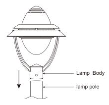
Step 3: Tightened the hexagon screws by hexagon wrench. Make sure until tihgtened
