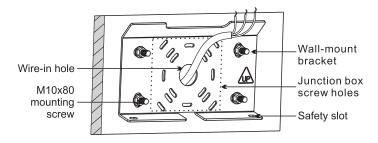
Secure the fixture by attaching a tether to the safety slot.
