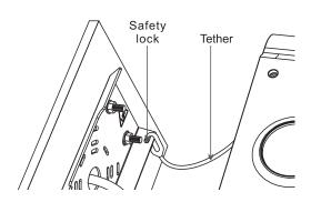
Release 2 allen head screws at the top of the gear box door.
