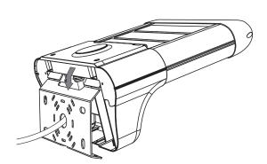
Make sure wires are inside the junction box and not pinched. Tighten 2 allen head screws on the bottom of the fixture.
