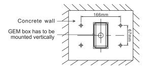
Put a power cable through wire-in hole. Use a spirit level to ensure lay horizontally and anchor wall-mount bracket to the concrete wall by using 4 mounting screws. (Bracket has to be faced upwards)
